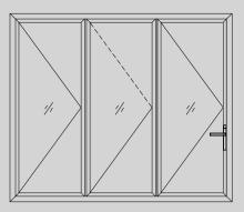
95 surface-mounted hinge, 3+0 configuration low-track external folding folding door
