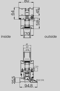
External folding low-track upper and lower positioning structure
