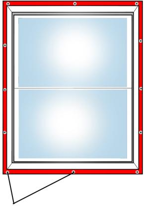
Screws are placed no less than 12" apart around the entire nail fin. Minimum 1 1/4" corrosion-resistant, pan head nails or screws needed.
